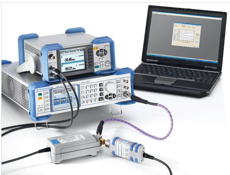
Calibration of an R&S®NRP-Z55 thermal power sensor.
